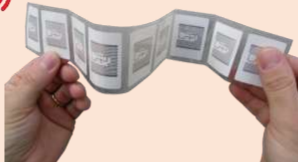
RFID UHF printable adhesive labels for asset tracking & inventory
